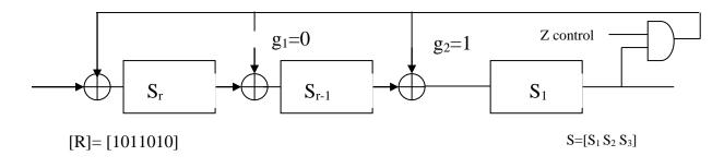
First we write the transition equations for  $S_1 S_2 S_3$  when Z=1 :-
